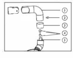
① lamp arm ② screw ③ decoration cover Connector Sconnecting shaft installation method: Connect the lamp arm, decoration cover
