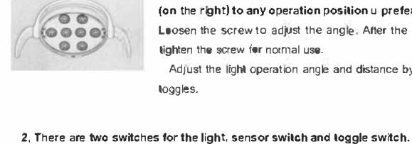
Loosen the screw to adjust the angle. After the adjustment, tighten the screw for normal use.
